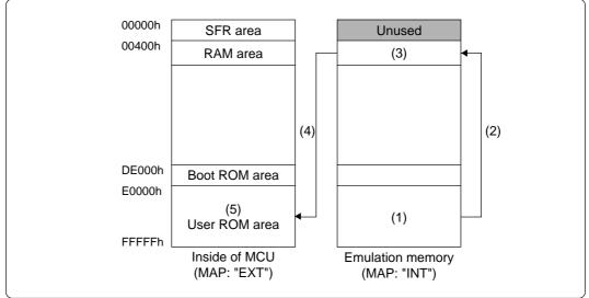
*Figure 4.2 Memory map when debugging in microcomputer mode*
